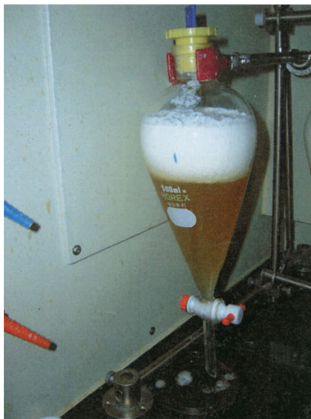
Figure 1 Photograph showing creaming process of skim natural rubber latex. [Color figure can be viewed in the online issue, which is available at www.interscience.wiley.com .]
